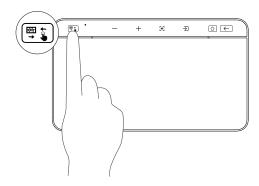
3 Put the TouchBoard back to the charging dock, wait for 10 seconds until the icons on the first row of the TouchBoard light up. Pairing is completed.
