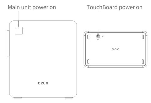
2 Long press on the upper left corner for 3 seconds until the LED indicator blinks in blue color.
