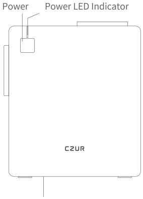
Elevation Bracket, 4°/8° Two-level Adjustment
